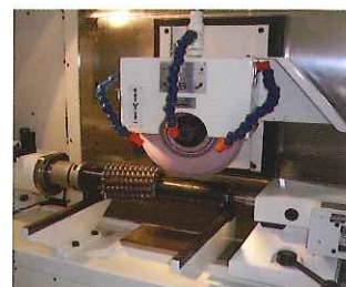
ホブの取り付けや砥石の交換が快適に行える 広い加工エリア Wide and large working area for comfortable set up.
